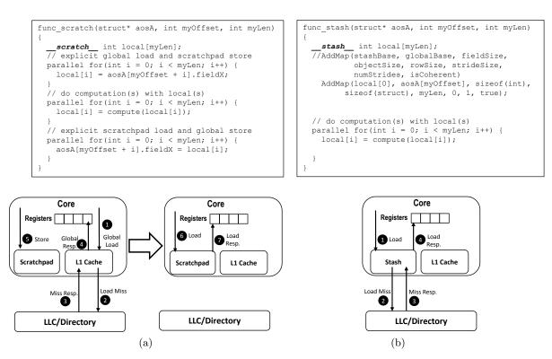
Figure 4.1: Codes and hardware events to copy data from the corresponding global address for (a) scratchpad and (b) stash (events to write data back to the global address are not shown).
