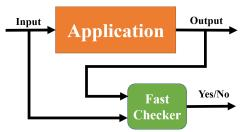
**Figure 1.** An approximate checker takes as input the input and output of an application, and checks whether an error occurred during execution.
