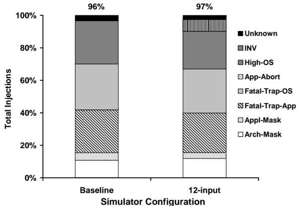
Fig. 2. Effectiveness of different symptoms to detect faults in various microarchitecture structures. Software-level invariants improve the coverage of SWAT detection from 96% to 97%.
