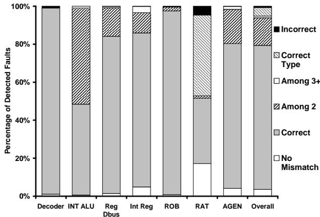
Fig. 1. Effectiveness of microarchitecture-level fault diagnosis. The figure shows the ability of the diagnosis algorithm to accurately diagnose detected faults. On an average, 96% of the detected faults are accurately diagnosed.
