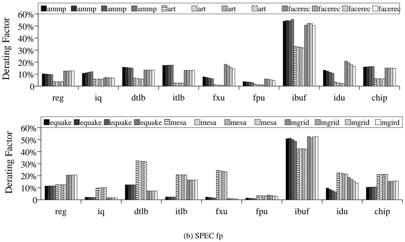
**Figure 2. Architectural derating factor for each structure (a) for SPECint and (b) for SPECfp benchmarks. Note that the scales on the two graphs are different. For each application, the four bars in a graph represent the four technology generations, going from 180nm to 65nm.**
