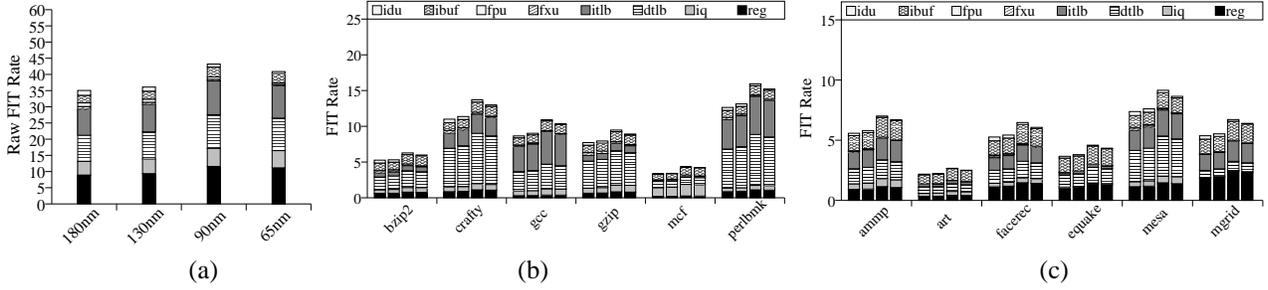
**Figure 1. FIT rates (a) for raw errors, (b) with architecture masking for SPECint benchmarks, and (c) with architecture masking for SPECfp benchmarks.**
